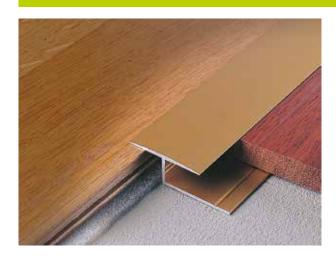
WOODTEC LG profiles are specifically designed to join two adjoining floating wood floors. The size and shape of the profile section allows for differential movement typical of wood flooring. Its smooth top surface fits under doorways making it perfectly suitable for thresholds.
